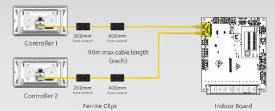
Ferrite clip, if supplied, should be placed approx. 200mm and 400mm from the NEO.
