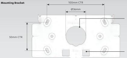
Please note that there is a return lip on the rear of the bracket. A 38mm hole will need to be drilled for clearance in order for controller to recess.
