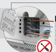
Use Rear hatch as tool to de-press terminal while feeding wire
