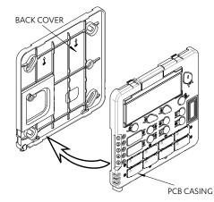
6. Attach the front cover, as shown in the diagram below IMPORTANT
