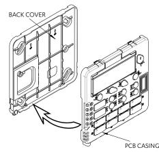
6. Attach the front cover, as shown in the diagram below
