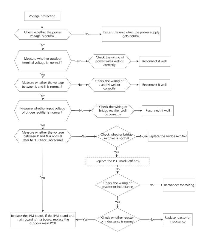
Note: For certain models, outdoor PCB could not be removed separately. In this case, the outdoor electric control box should be replaced as a whole.
