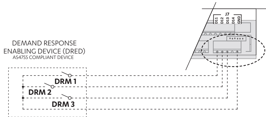
DRM CONNECTION DIAGRAM (See the Electrical Wiring Diagram Provided with the unit for details)
