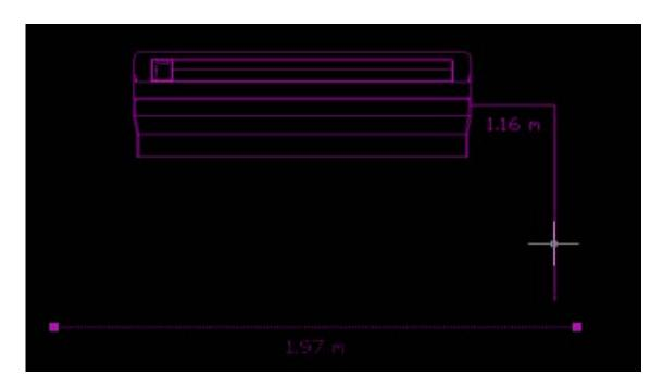
Click on the pipes that you want to join together and right click to put the joint in place as is shown in the picture below.
