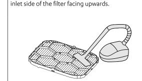
Clean the filter with a vacuum cleaner, with the air
