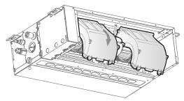
Slanting downward, remove the lower propeller housing.
