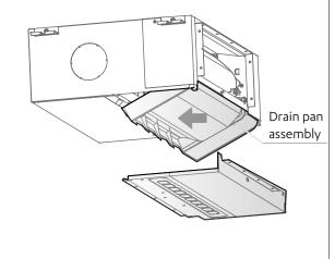
(4) Shift the drain pan downwards until the drain pan is removed from the unit body
