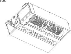
Remove the motor and wind wheel together; unscrew the screws securing the wind wheel in place and remove the wind wheel and motor.
