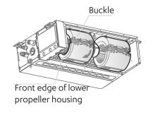
Slanting downward, remove the lower propeller housing.
