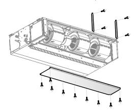
Refer to the maintenance previous of fan casing to remove the lower fan casing located at the side with a coupling and loosen the fastening screws on the coupling.
