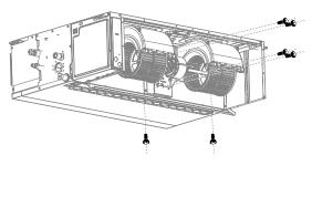
(5) Remove the motor and wind wheel together.
