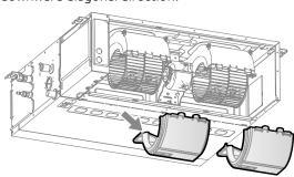
Loosen the screws on the upper propeller housing.
