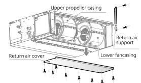
2 Remove the three screws, plate the approximately 30 degrees, as shown in the figure.
