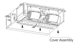
(3) Remove the lower propeller housing in a downward diagonal direction.
