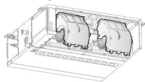
(7) Remove the upper fan casing.
