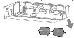
3 Loosen the two M5 screws attached to the middle cross member and the two M3.9 screws attached to the side panel and remove the bearing holder.
