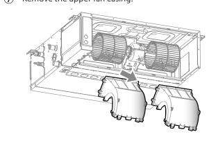
(8) Note: Installation notes are as follows: The slot and latch bolt, and the limiting groove and side wall edge should be aligned first, and then be fastened; Check whether the limiting groove, positioning rod and buckle are installed in place, and the limiting latch bolt shall enclose the outside of the fan casing.
