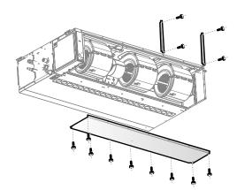
Refer to the motor shaft service procedure and remove the fan, connecting shaft, and coupling.
