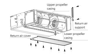
Remove the three screws, plate the approximately 30 degrees, as shown in the figure.
