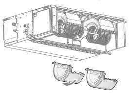
4 Loosen the four M5 screws on the motor holder and the fastening screws for the fan.
